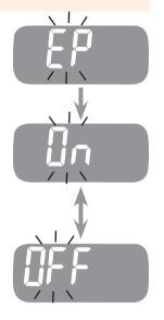
Note: If the pre-set expiration date expires, the meter will display the following. For example, in the case when the expiration date is set to October of 2017, the meter displays "EP" at the start of November of 2017.
