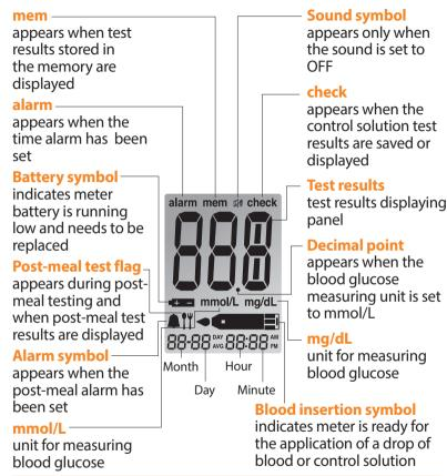
Note: It is recommended to check if the display screen on the meter matches the illustration above every time the meter turns on. Do not use the meter if the display screen does not exactly match the illustration as the meter may show incorrect results.
