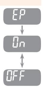
Note: If the pre-set expiration date expires, the meter will display the following. For example, in the case when the expiration date is set to October of 2014, the meter displays "EP" at the start of November of 2014.
