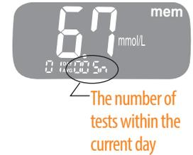
Use the **s** button to scroll through the test results, starting from the most recent and ending with the oldest. Press the **>>** to return to the results seen previously. The test date and the recorded temperature will display alternately. After checking the stored test results, hold the **s** button to turn off the meter.
